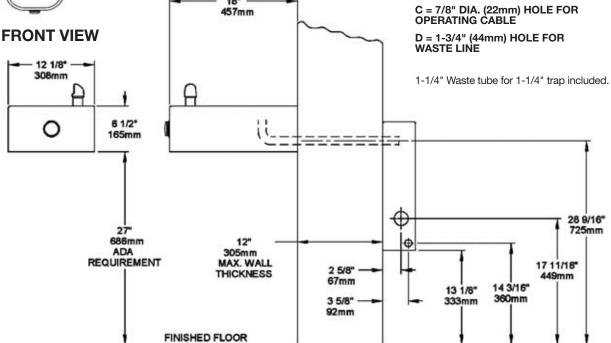
Note: A service supply stop (not included) must be installed at the fountain inlet line. Important: Freeze-resistant box must be installed on interior non-freezing wall.
